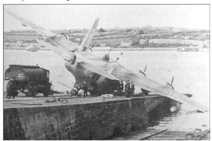
The reason for the subsequent transfer of ML 743 to 201 Squadron for October 1944, was that this aircraft had been repaired following the accident which occurred with 461at RAF Pembroke Dock: For on the 28th. May whilst on a slipway ML 743 (in process of being launched) had been damaged owing to the collapse of the beaching chassis' leg. Major repairs were conducted under the auspices of No. 43 Group of RAF Maintenance Command.
